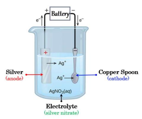
Applications: Used for jewelry, cutlery, electronic components, and in corrosion-resistant coatings.
