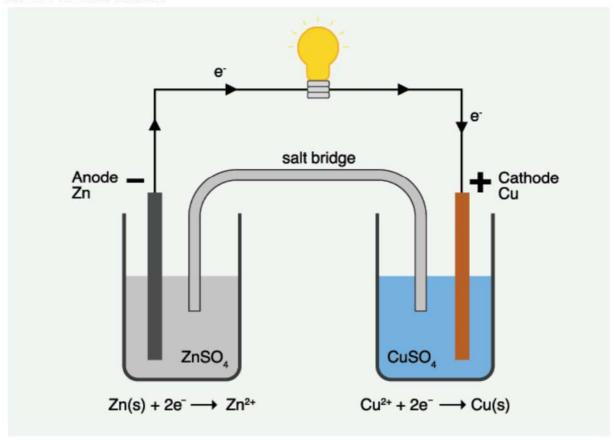
Oxidation: Loss of electrons at the anode. Reduction: Gain of electrons at the cathode.
