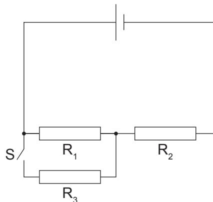
What is the power dissipated by  $R_1$  when S is closed?
